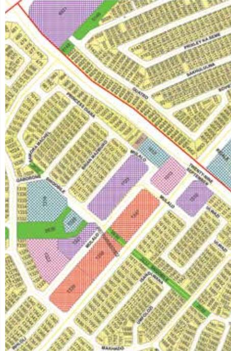
Photo 2: Survey and land use plan (zoning scheme) of Ivory Park. Note the misalignment between the plan and actual settlement.
